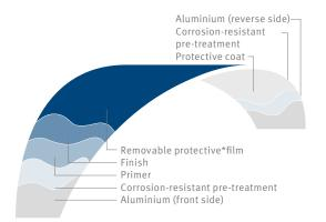
\* Please remove the protective film immediately after mounting of the panels and do not expose the protective film to UV radiation for a longer period of time, not even during storage. The BEMO-FLON PROTECT paint system offers a very wide range of colours, a large variety of possible gloss levels and is available with differently structured surface finishes. BEMO-FLON PROTECT is our recommendation for an economical, durable and easy-toapply paint system outside highly corrosive areas.
