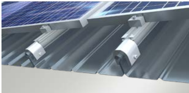
PV modules can be mounted on BEMO standing seam roofs without any drilling through with the BEMO-AKKORD rails.
