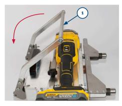
**1. How to open the seaming machine:** Turn the lever (1) down.
