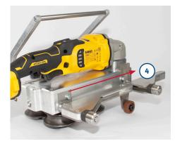
**4. Closing AKKORD machine:** The tension slide (4) need to be closed.
