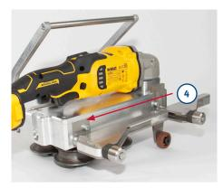
2. Preparation AKKORD machine: To allow for a wider opening the tension slight (4) needs to be unlocked.
