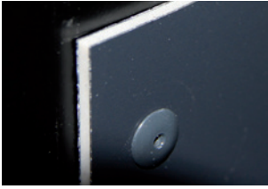
normal cutting edge visible plastic core
