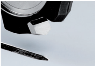
V-grooving milling cutter for the composite milling machine PF 1200
