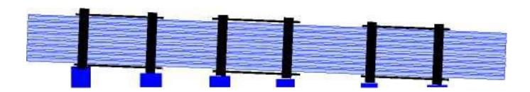
When storing packed profiled panels on the roof of the building, take its load-bearing capacity into account.
