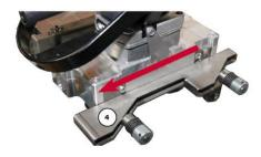
**2. BEMO-TOP & AKKORD machines** For these machines, the tense slide (4) must also be opened to allow the necessary attachment width.
