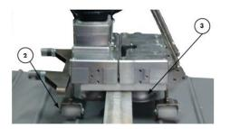
**3. Place the seaming machine on the flange** First, the seam must be folded around 300 mm with the manual folding pliers. Place the machine in the open position over the flange so that the support rollers (2), setting the height for the 50s and 65s profile possible, sit up and the forming rollers (3) enclose the flanges.
