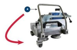
**1.** How to open the seaming machine: Turn the lever (4) to the left side.
