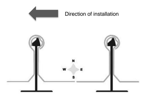
In this example, installation work proceeds from right to left – against the direction of the main airflow.
