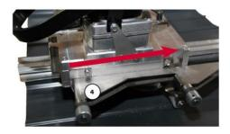
**4. BEMO-TOP & AKKORD machines** For these machines must first the tense slide (4) closed (pushed back).
