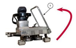
**5.** How to close the seaming machine: Turn the lever (4) to the left side.
