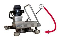
**1.** How to open the seaming machine: Turn the lever (4) to the right side.
