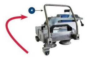
**3.** How to close the seaming machine: Close the lever (4).
