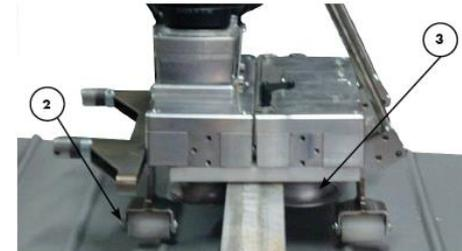
**3. Place the seaming machine on the flange**
